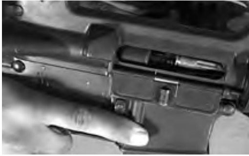
Figure 3-15. Brass Obstructing the Chamber.
